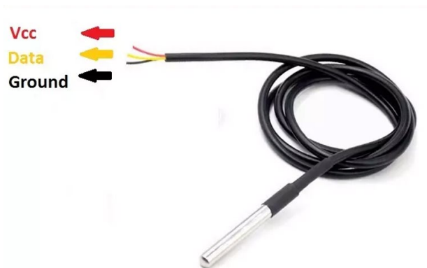
Slika 35 DS18B20 raspored pinova
